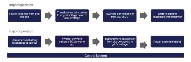
The physical operation of an asymmetrical project, or the "net export" element of an ESS Project is to generate power and then export it. This is illustrated in the diagram below.
