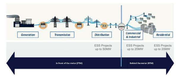
An ESS Project's point of connection can vary by location and voltage; however, they are broadly either connected in front of the meter (i.e. a project has its own point of connection) and imports
