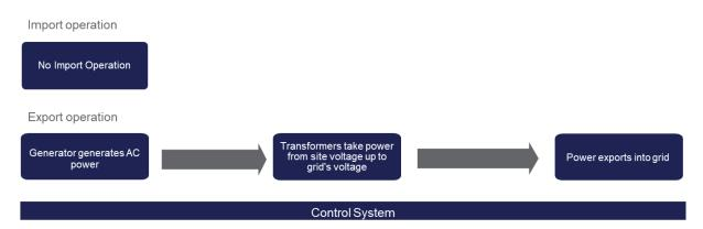
One important feature of an ESS Project is the project-level control system. This control system monitors the individual physical elements of the ESS Project site from a safety and functional perspective to make sure it can instruct the project to operate according to the project's contractual requirements. As the control system can be monitored remotely, projects are unmanned most of the time and are mostly accessed only for preventative or reactive maintenance, as required.
