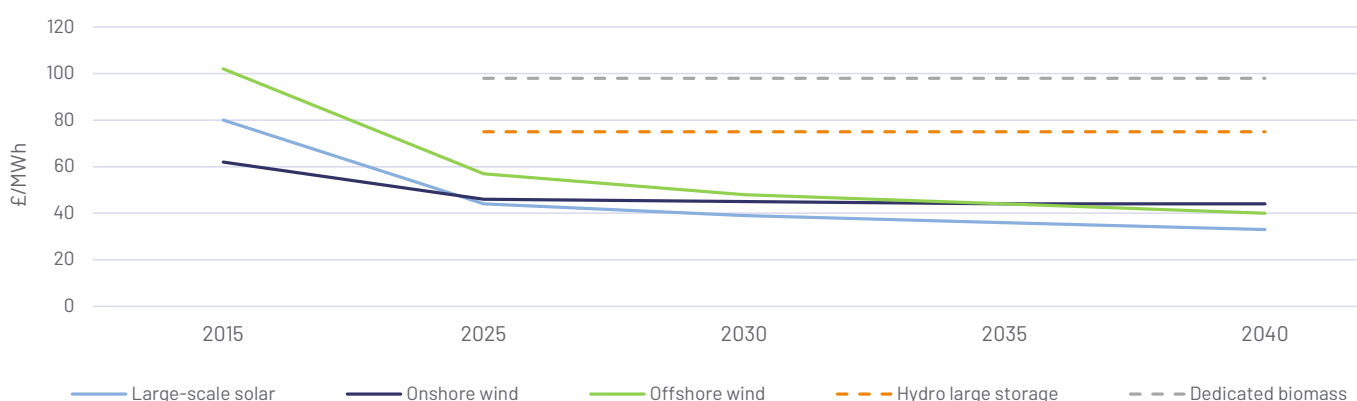
Figure 2: LCOE Forecast (£/MWh) 11
